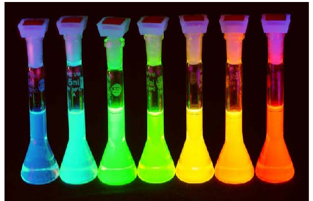
Image of fluorescence in various-sized Cadmium Selenide Quantum Dots.
