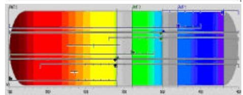
as small as 50nm. The images above represent fluorescent emission wavelengths that can be separated into 3nm blocks using Bio-Rad's LaserSharp2000 software package. Fluorochromes, e.g. Fluorescein and GFP, which have overlapping emissions, can be viewed independently of one another.
