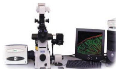
BioRad Radiance Rainbow system equipped with inverted microscope configuration
