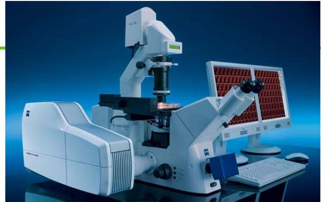
movement of intracellular molecules in ultra-fast processes such as cell adhesion, cell motility and cell signaling. The combination of the microscope's CCD line detector, zoom optics, and ultra fast Z-drive permit the user to obtain 3D images stacks every second.
