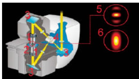
Diagram of Leica's 4Pi Microscope.
